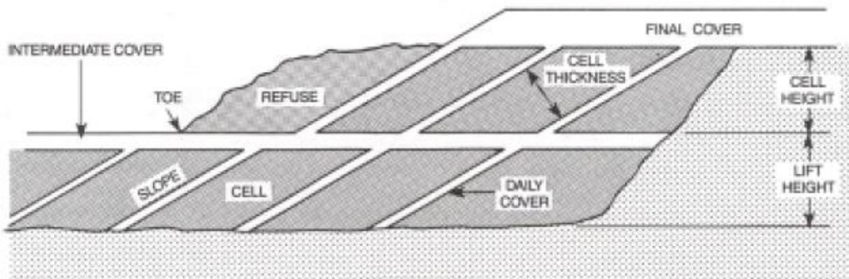
Figure 0.3: Typical Landfill Cell Construction<sup>4</sup>
