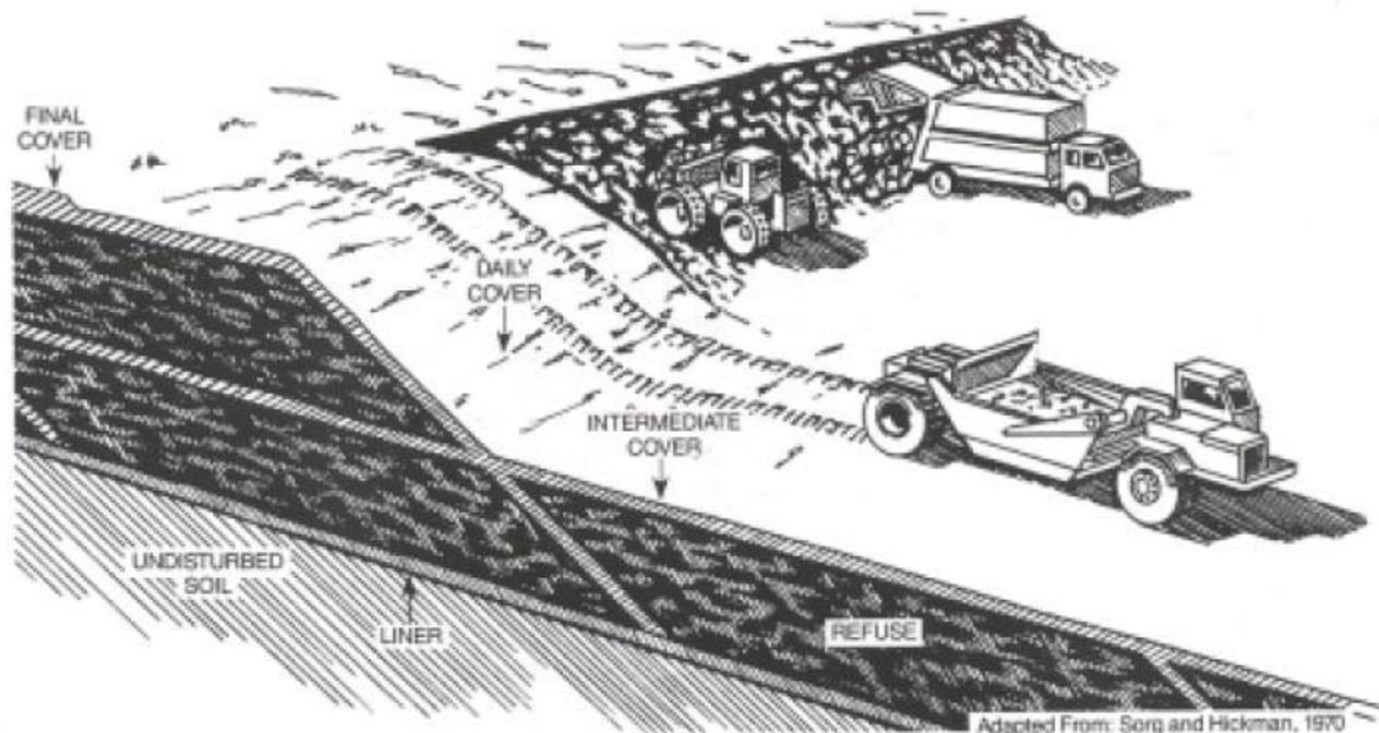
Figure 0.1: Area Method of Landfilling<sup>2</sup>
