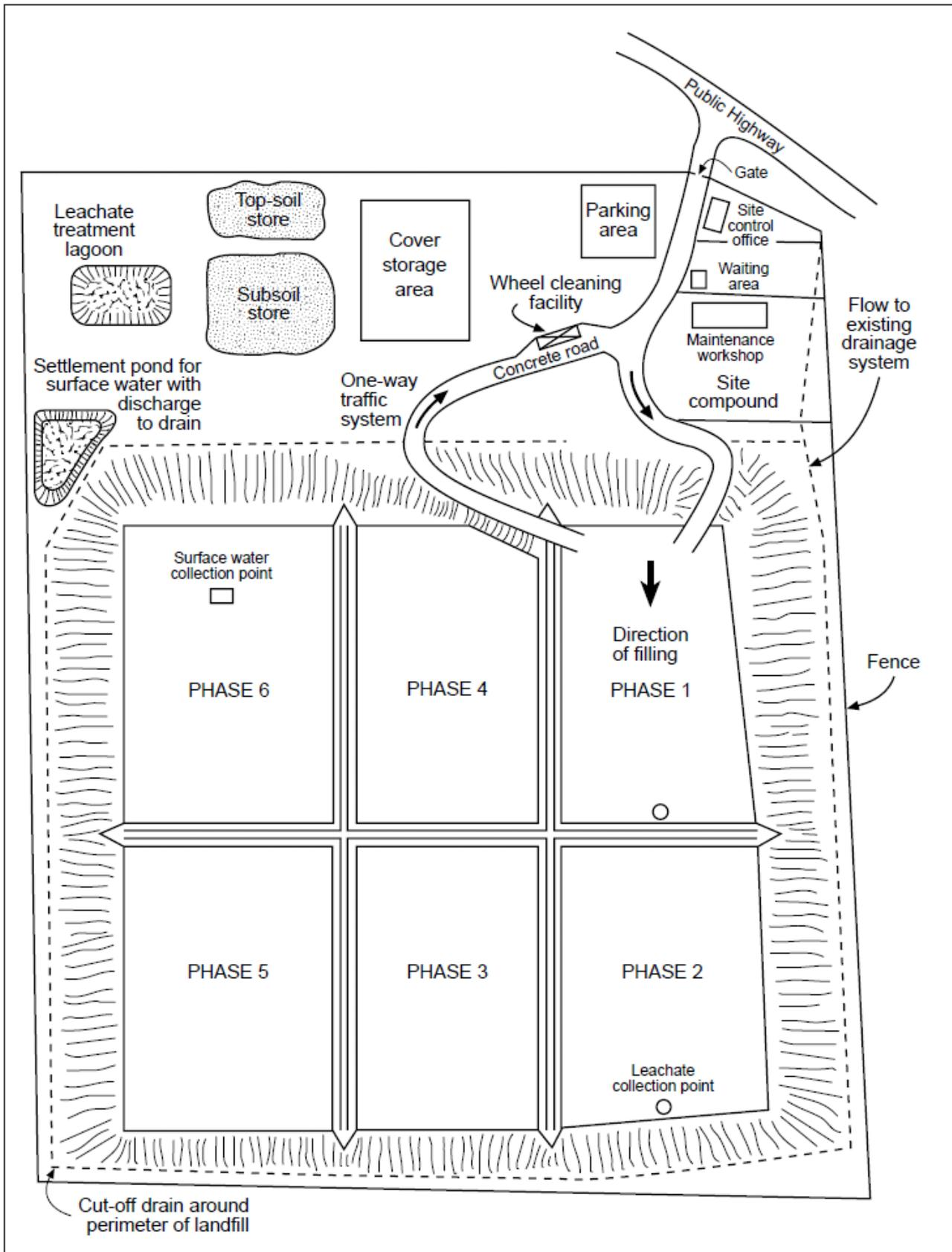
Figure 0.4: Typical Operational Plan for a Landfill Site<sup>5</sup>
