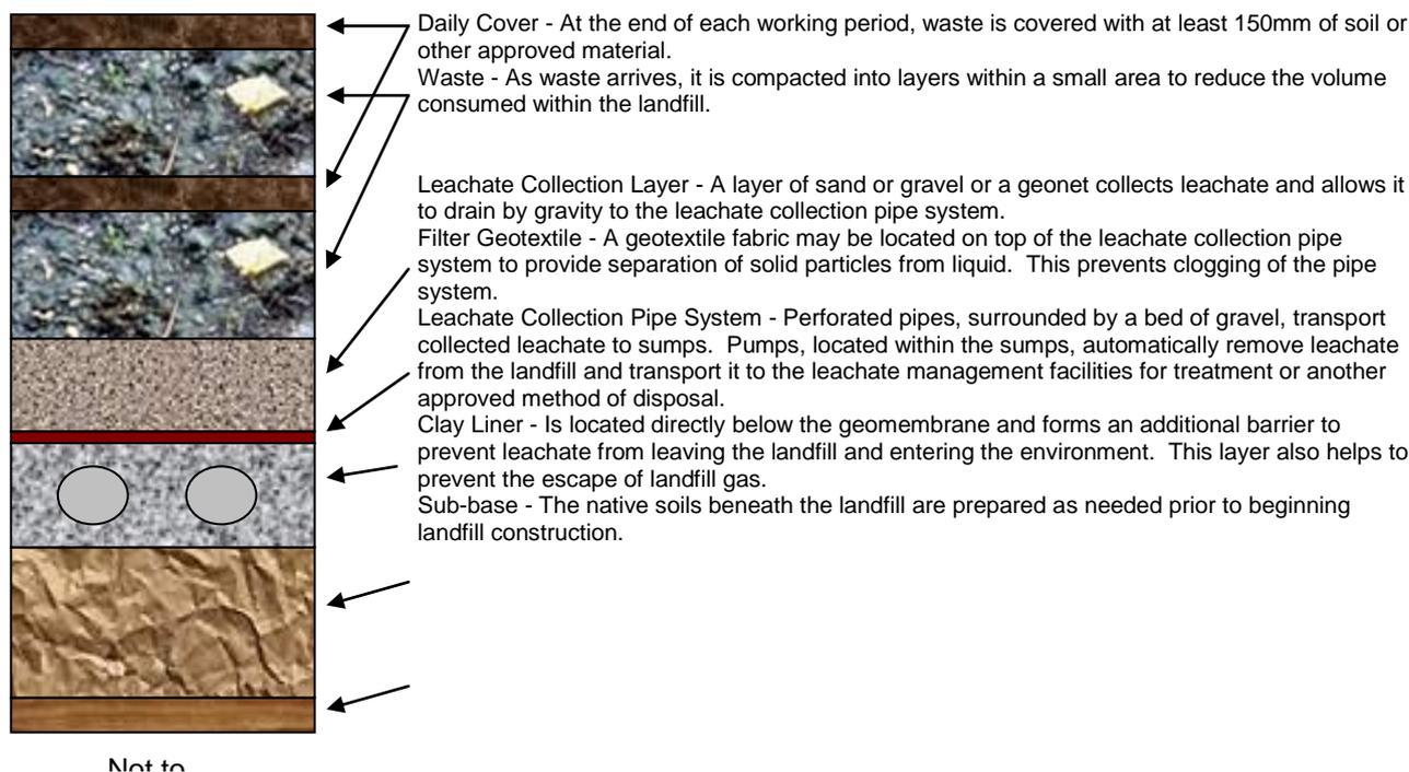
**Figure 0.5: Single Liner System**
