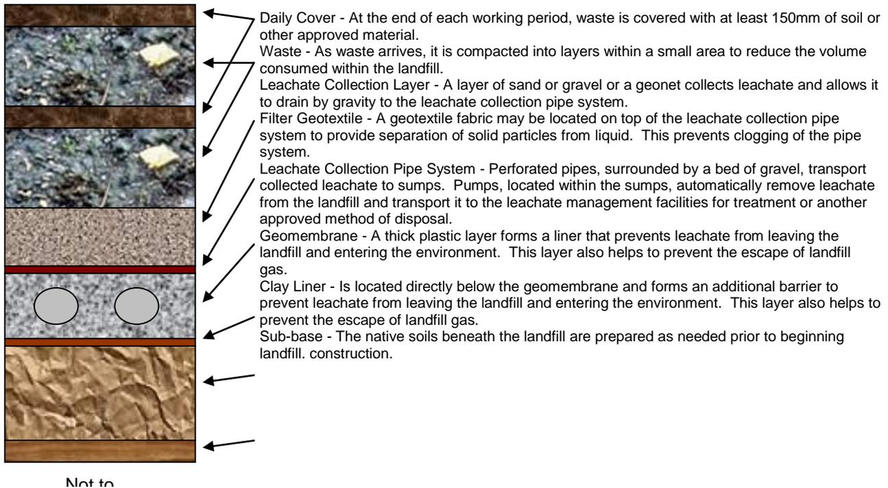
**Figure 0.6: Composite Liner System**
