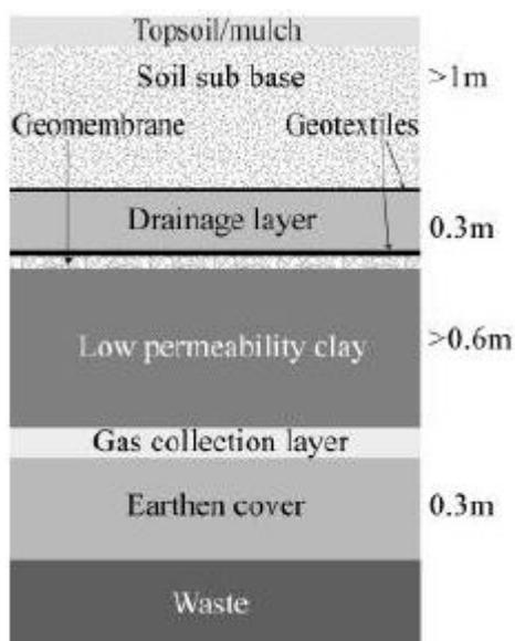
**Figure 0.2: Indicative Landfill Cap Design<sup>7</sup>**
