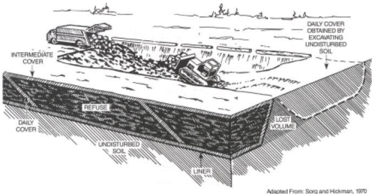
Figure 0.2: Trench Method of Landfilling<sup>3</sup>
