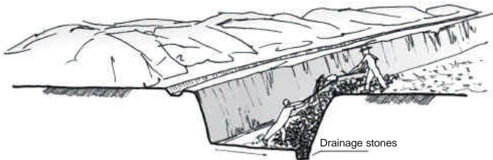
Figure 7.30 MSW is raked down into the trench and leveled
