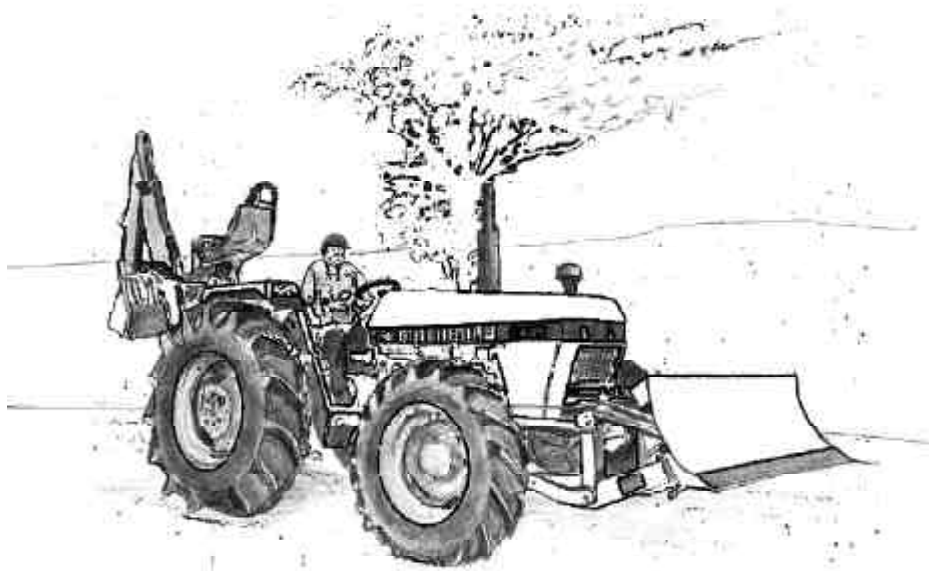
Figure 3.3 Farm tractor adapted for sanitary landfill operations
