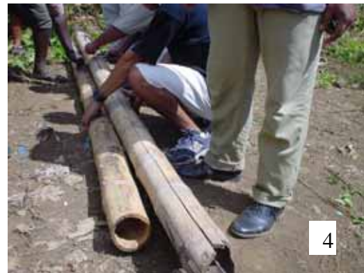
Photo- 15: Bamboos as Substitute Material for Pipes
