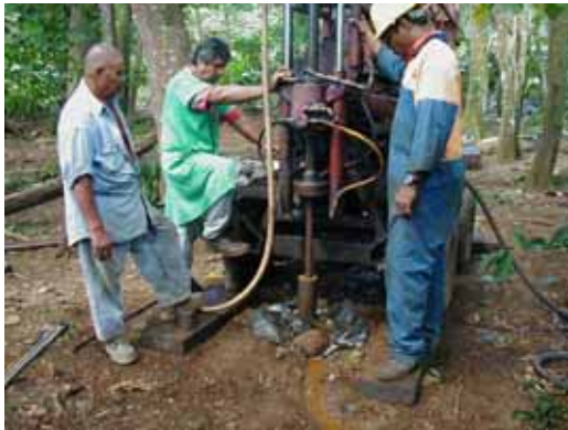
Photo- 3: Site Investigation (Exploratory Boring and Topography Survey)
