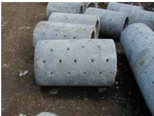
Photo- 14: Leachate Collection Pipe
