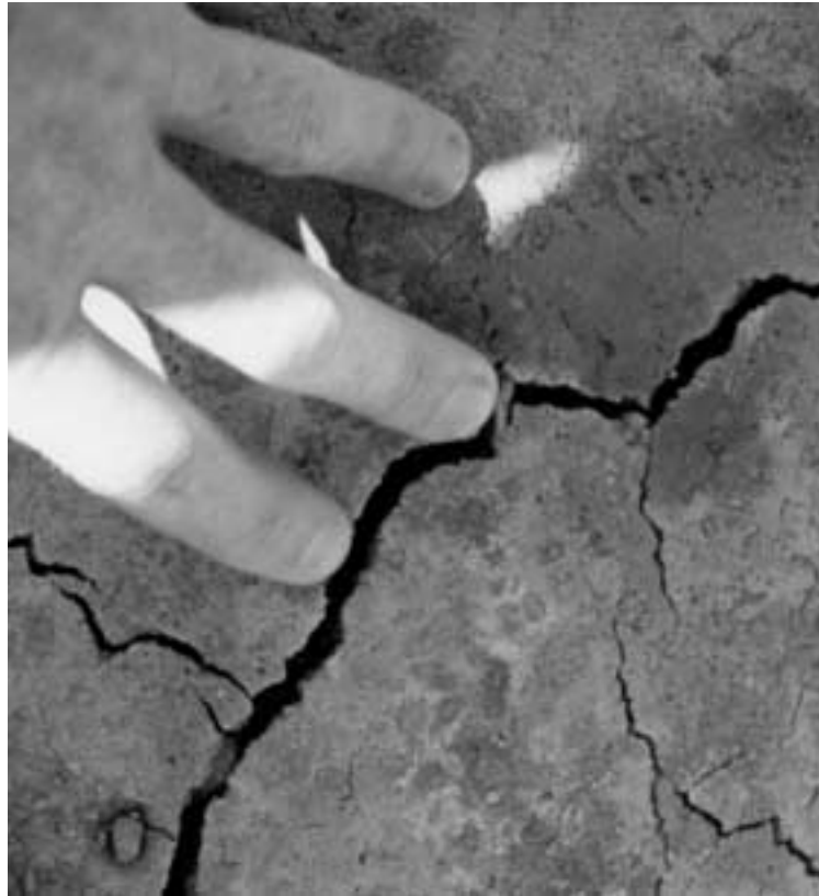
Figure 3.4. Desiccation Cracking in Subtitle C Cover Barrier Layer (15 minutes after compaction)
